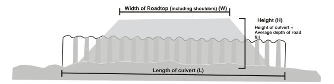
Determining the length of a culvert:
